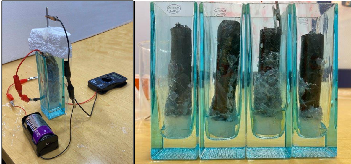
Figure 9. EPSA Prototype (Left), Pipe Segments A, B, C, and D (Right)
