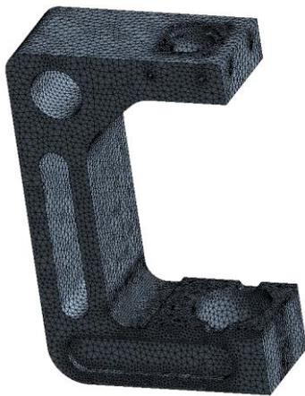
Fig 11. Optimized C-frame meshing.
