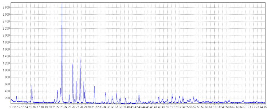
Fig. 4. Diffractogram of sulfur nanoparticles, obtained by using X-ray diffractometer
