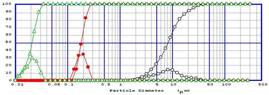
Fig. 2. Integral and differential distribution curves of ground in a roller mill and the resulting release of calcium polysulfide.
