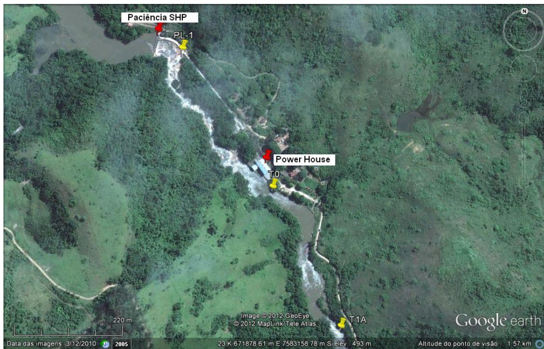
Figure 5 – Release point (PL-1) of the sediment marked with tracer and detection stations (T0 e T1A) in the experiments done in October 2012
