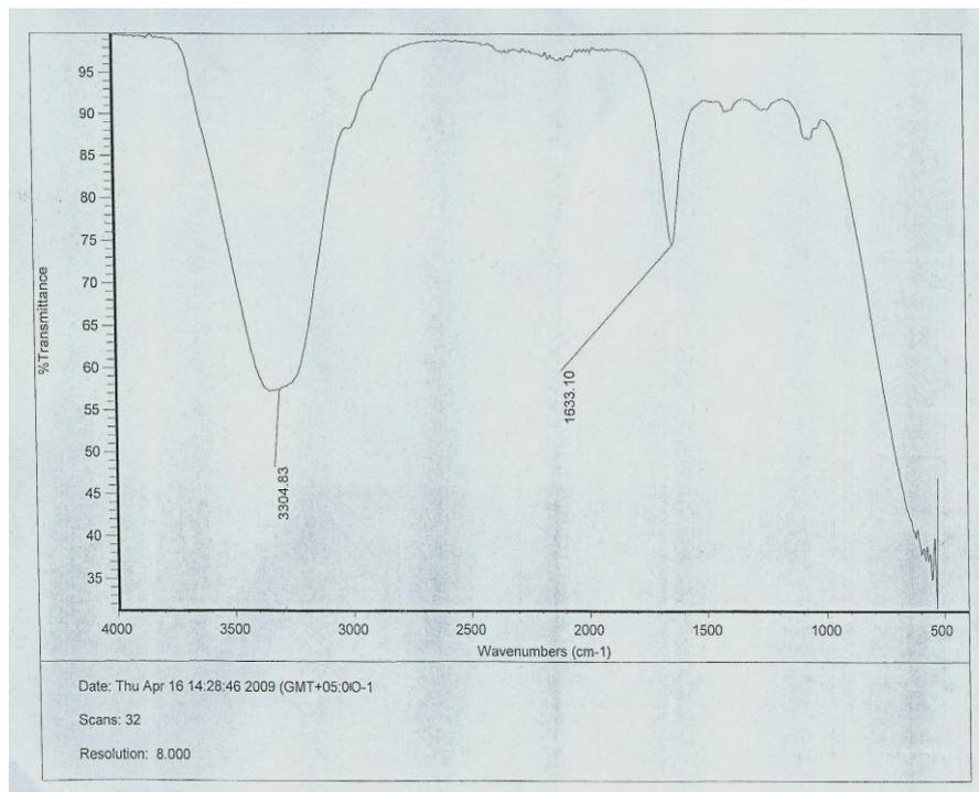
**Figure 4: FTIR Spectrum of bio oil sample**
