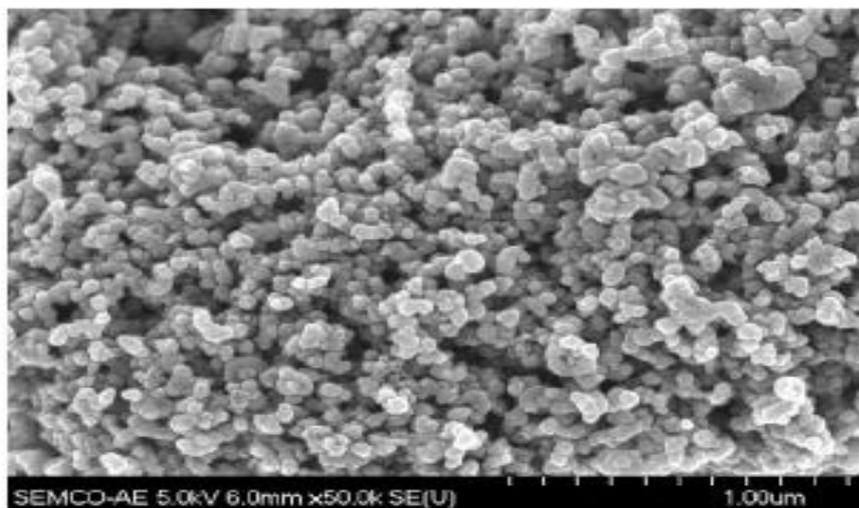
**Figure 5 SEM of cobalt oxide nano particles before gasification**
