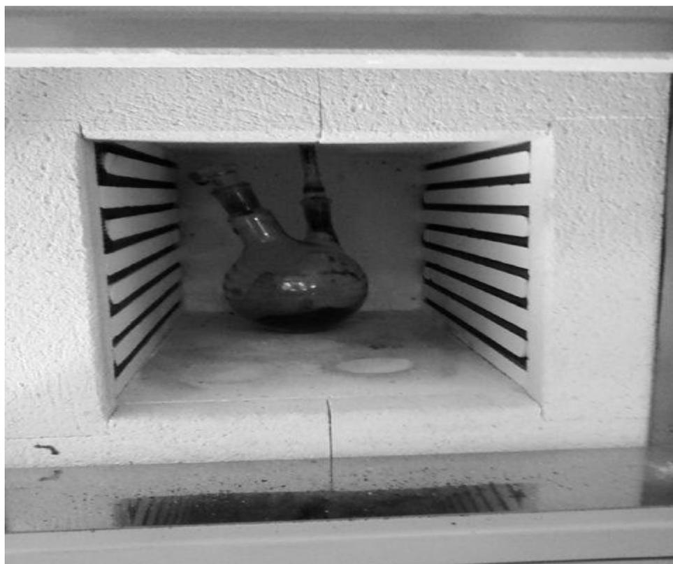
**Figure 2:** Flask with burning ash placed in the center of furnace
