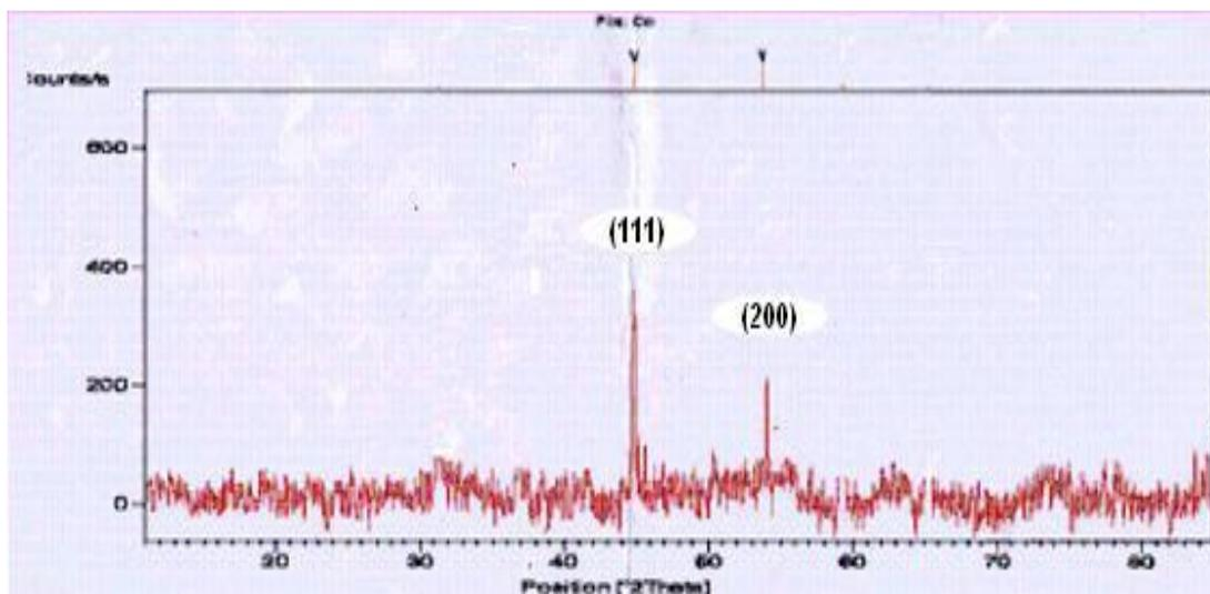
Figure 3: XRD Spectrum of Cobalt oxide Nano particles
