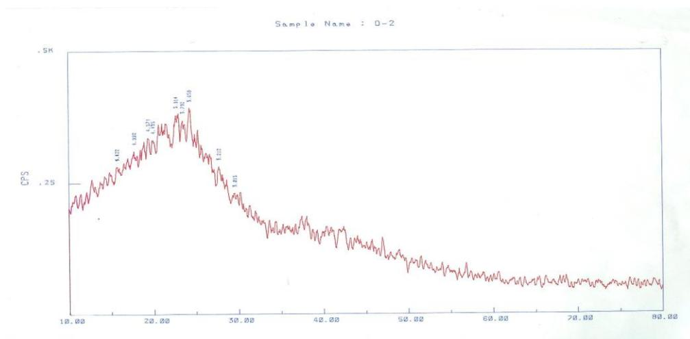
**Figure 7:** X-ray diffraction patterns of Char/Charcoal particles
