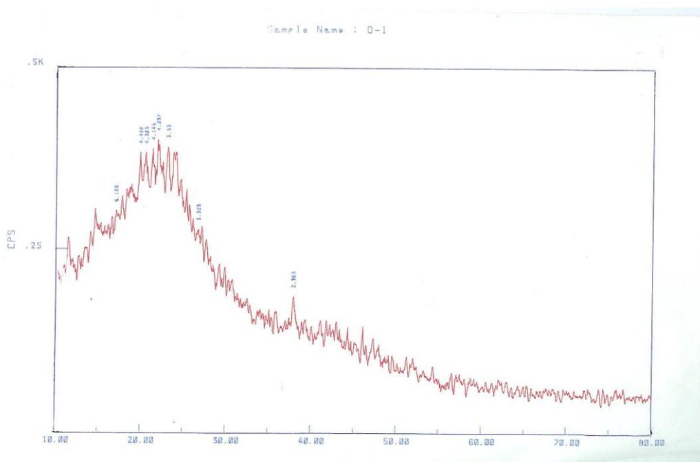
**Figure 6:** X-ray diffraction patterns of Char/Charcoal particles
