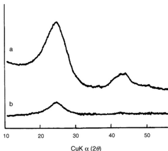
**Figure 9:** The XRD pattern of the carbon nano coils (a), compared to XRD pattern of carbon microcoils (b).
