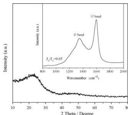
**Figure 10:** The XRD pattern and Raman spectrum (inset) of C<sub>R</sub>-600
