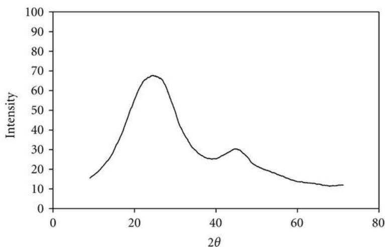
**Figure 8:** XRD Pattern of the spring like Multi Wall Carbon Nano Fibers.
