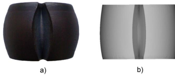
Fig. 2 Shape of deformed test sample at temperature 700 °C a) laboratory experiment b) computer simulation
