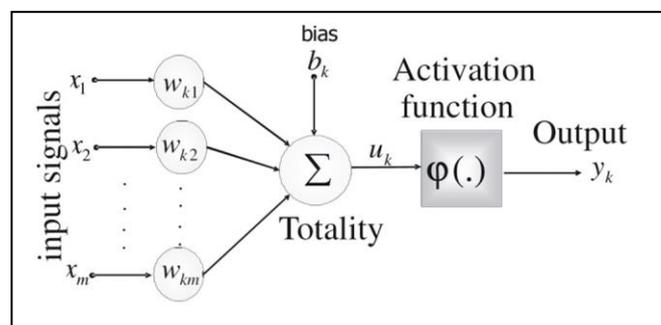
**Figure 3** – The artificial neurons structure used in ANN. Adapted from Haykin (2001).
