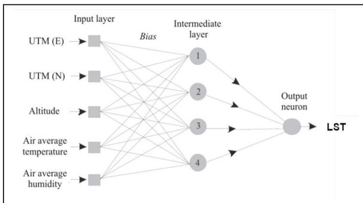
Figure 4 – The neural network structure used in the modeling of LST
