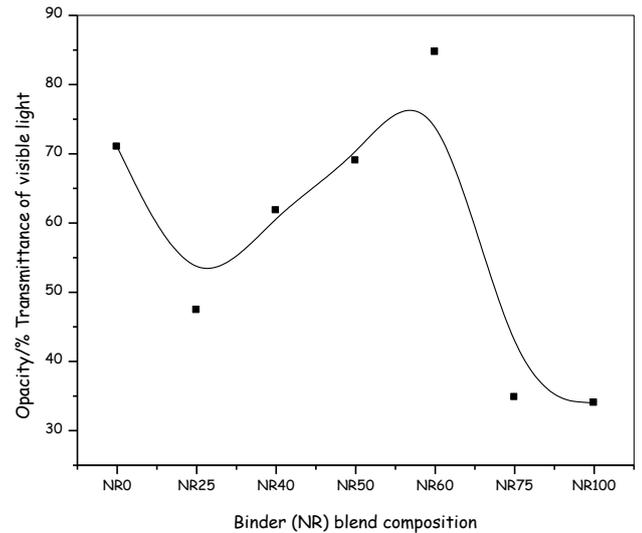
Fig.3. Opacity against paint's binder composition
