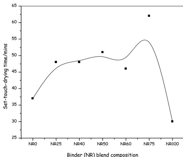
Fig.5. Set-to-touch drying time against paint's binder composition
