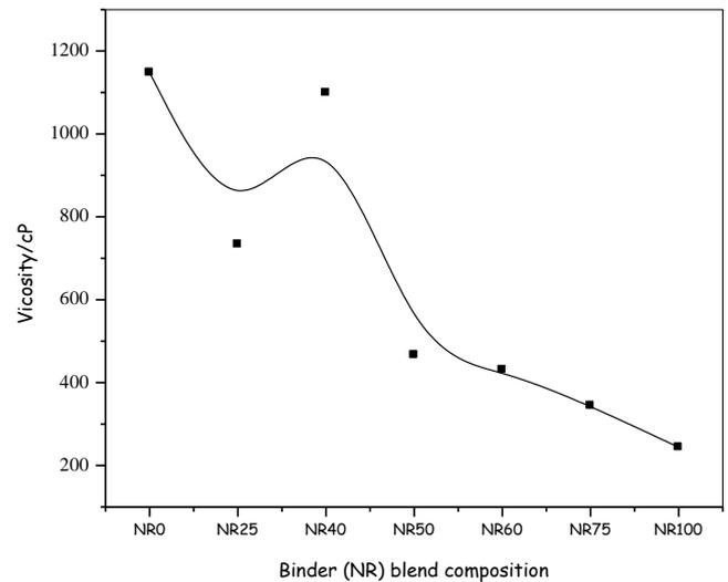
Fig.4. Viscosity against paint's binder composition
