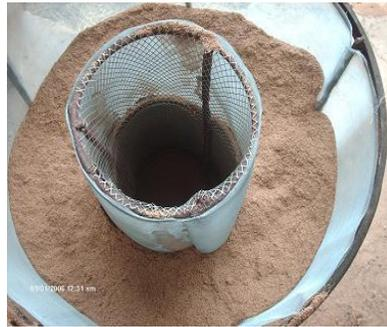
Plate 1. Filling the incinerator with rice husk.
