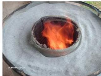
Plate 2. Rice husk incinerator charged with red hot Charcoal.
