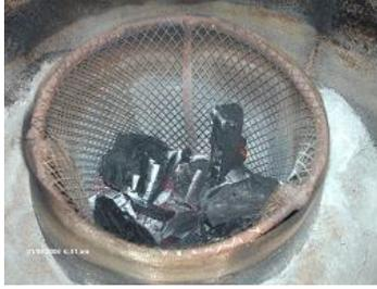
Plate 3. A close view of the incinerator converting rice husk to RHA.
